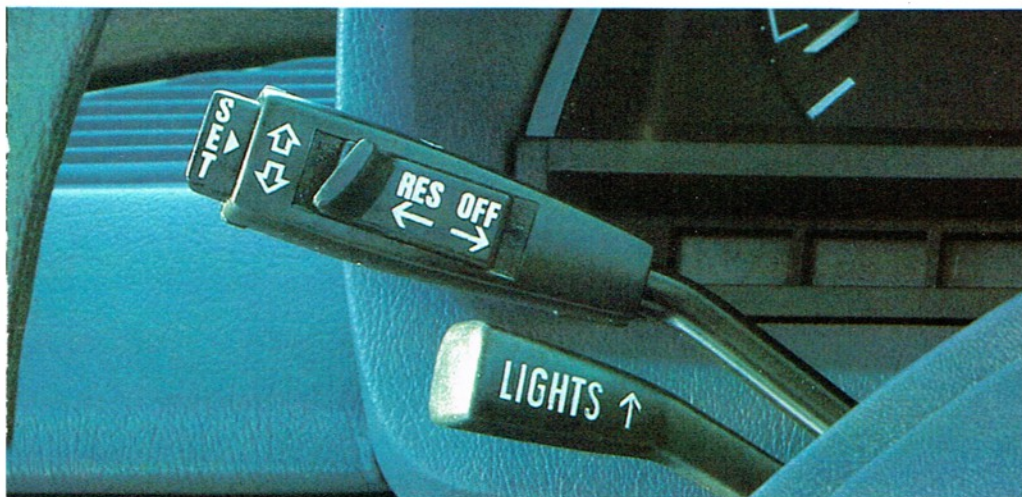
Above: cruise control, turn signal indicator, headlight dimmer, flasher stalk. Below: Headlight control stalk.
