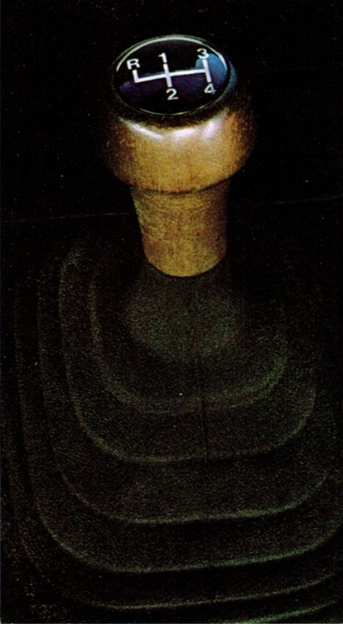
Four-speed fully synchronized manual transmission.
