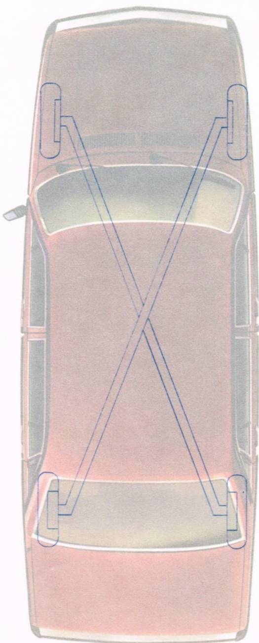
Two separate brake circuits are linked diagonally for directional stability in the event of a failure in one braking circuit.
