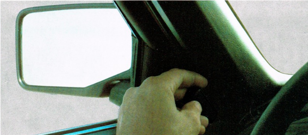
Tinted side view mirror is adjustable from inside.
