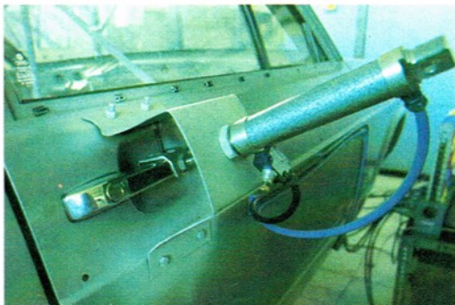
Doors are opened and closed thousands of times to simulate use.
