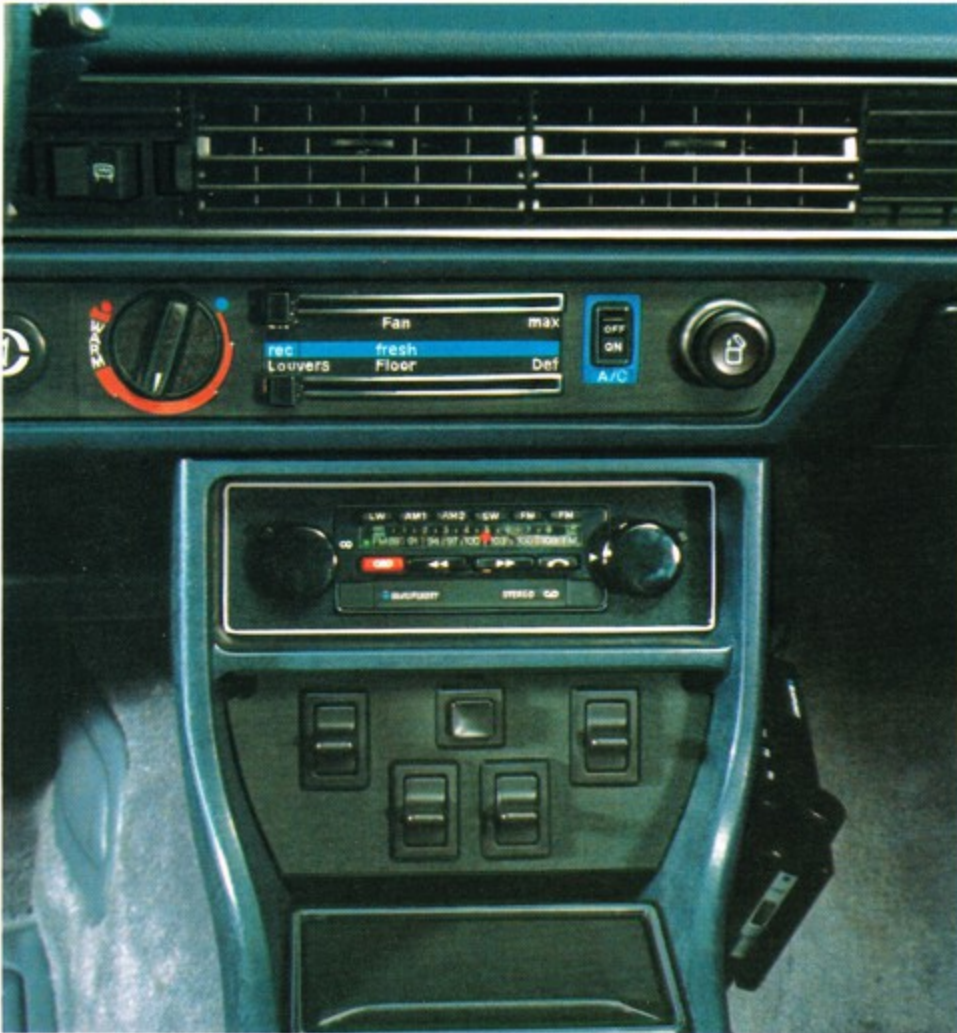
Air conditioning controls.
