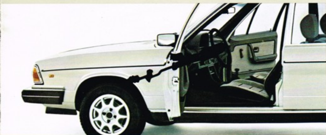
To reduce chances of injury, the steering wheel and column are designed to absorb energy on impact.
