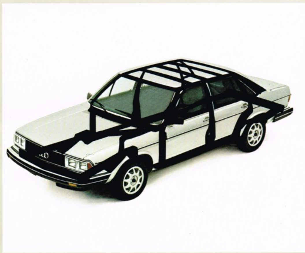
A "safety cell" is formed around the car's passengers by body components utilizing unitized construction for exceptional strength and rigidity.
