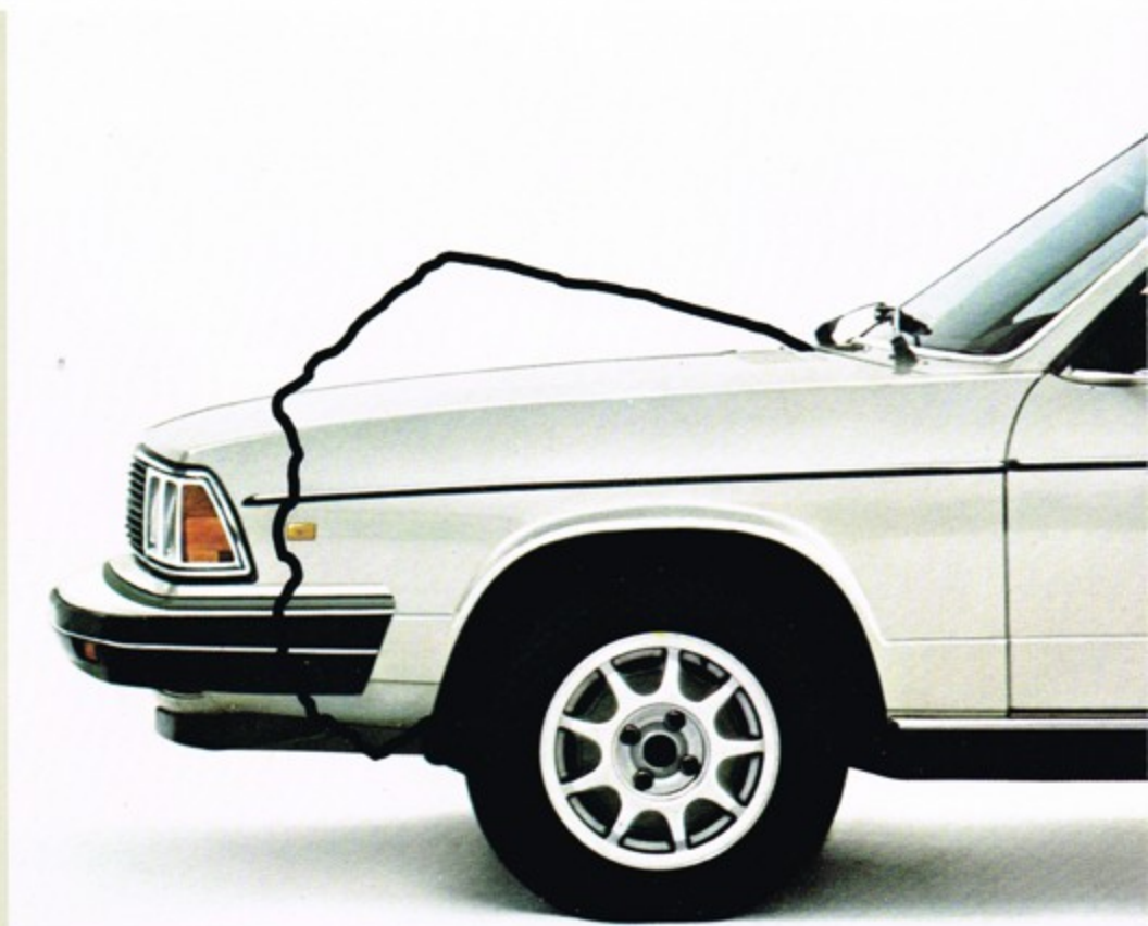
To protect the integrity of the passenger compartment, both the rear end and front end are designed to collapse at a controlled rate.
