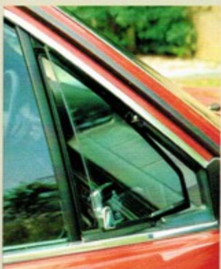
Front vent windows.
