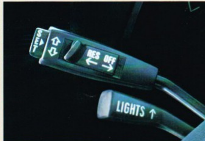
Several functions are controlled by the large and small stalks on the steering column.
