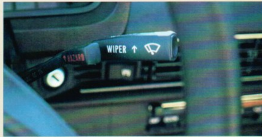
Stalk controls 2-speed wiper/washer, and intermittent wipe cycle.
